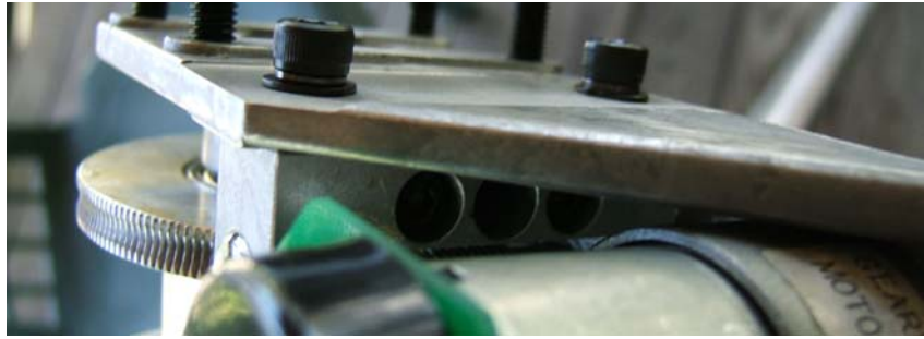
RA worm gear adjustment location. Yes, it's buried.
