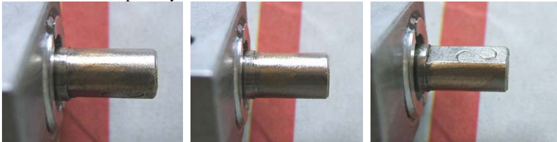
File marks galore, unequal filing, and an indication that the gears were put on and removed once before I received the mount
