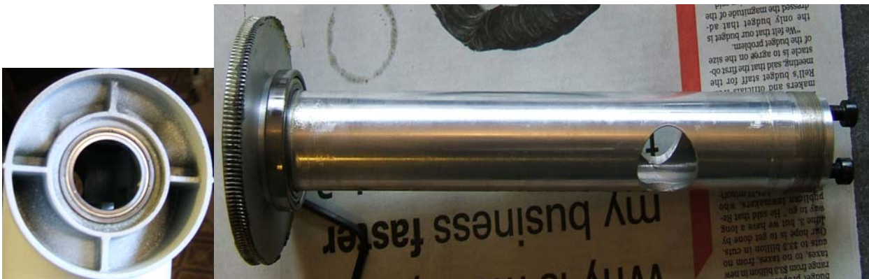
Top bearing in the Dec housing, and the bottom bearing on the Dec drive shaft
