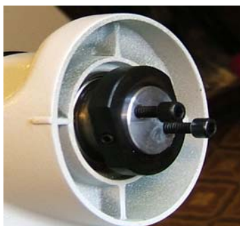
Dec shaft locking ring loosened with the saddle mount collar removed
